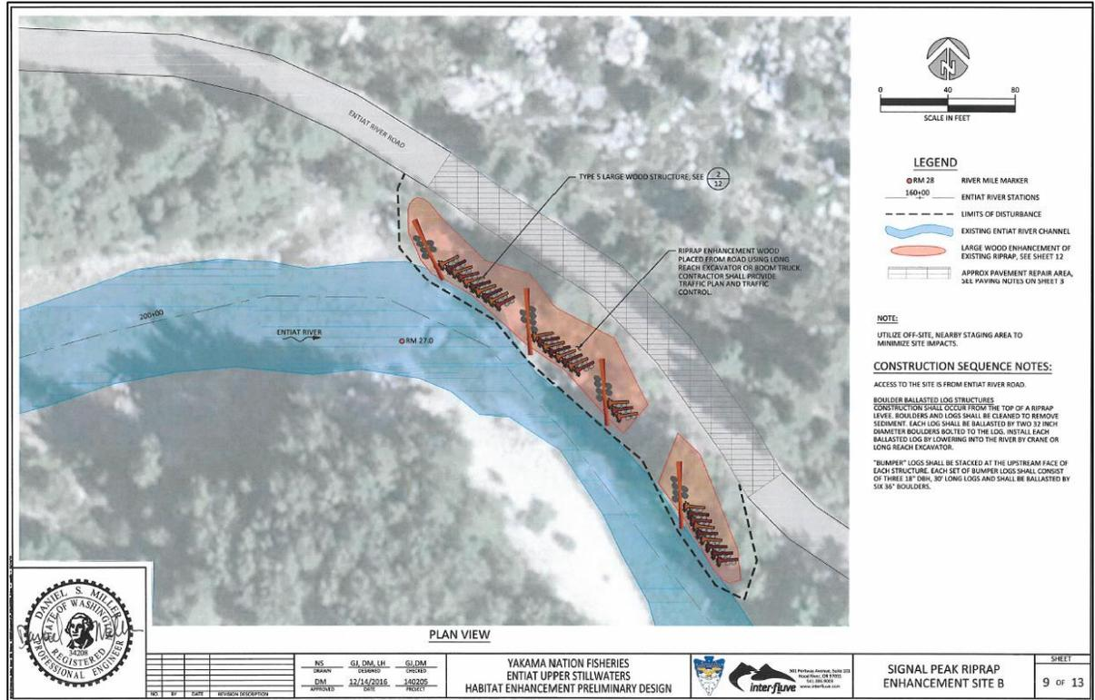
Figure 6. Signal Peak Riprap Enhancement Site B Design
