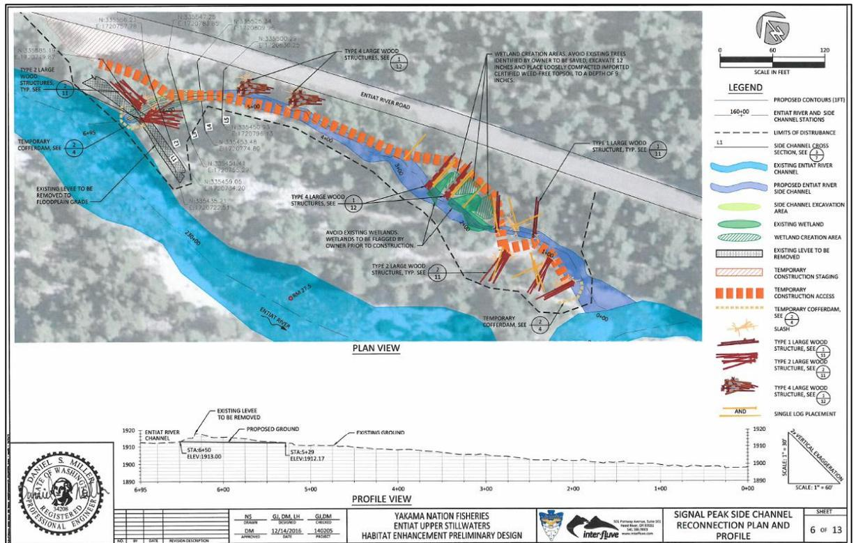
Figure 8. Signal Peak Side Channel Reconnection Design
